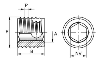
Female thread A = M6= 12 Length B Male thread E = 10 Min hole depth blind hole = 15 Min material thickness = 12 = -SW
